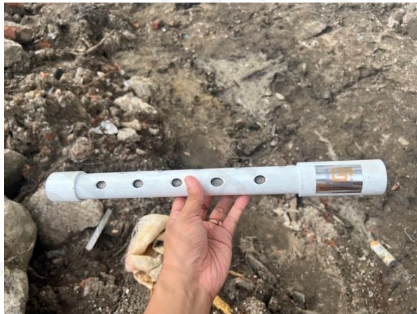
Figure 31: Casagrande Piezometer & VW Piezometers
