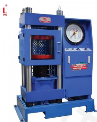
Figure 86: Concrete Compressive Strength Testing
