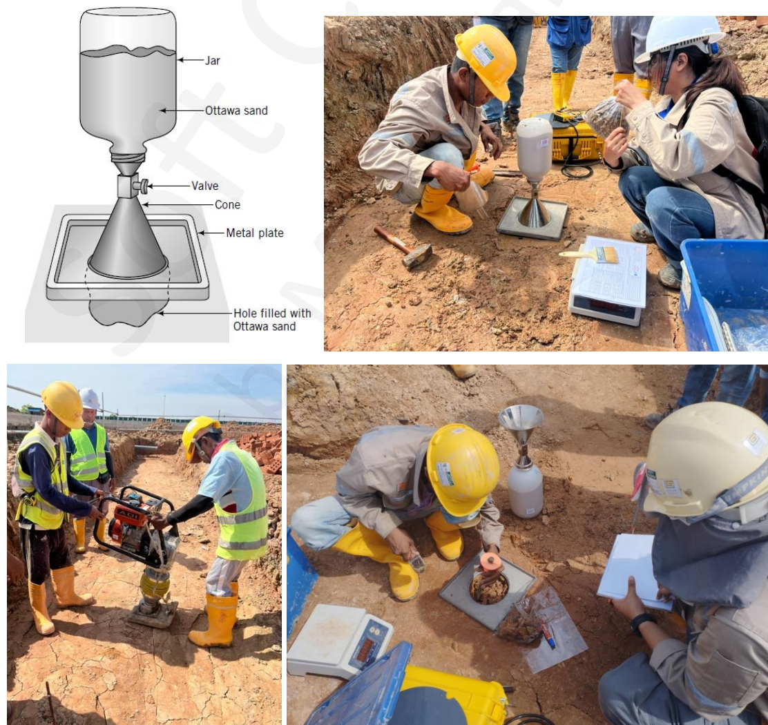
Figure 83: Sand Cone Test Equipment & Testing Photos
