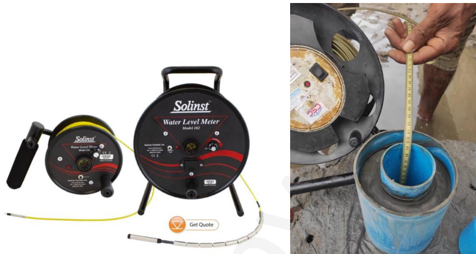
Figure 30: Water level meter and BH water level Measurement
