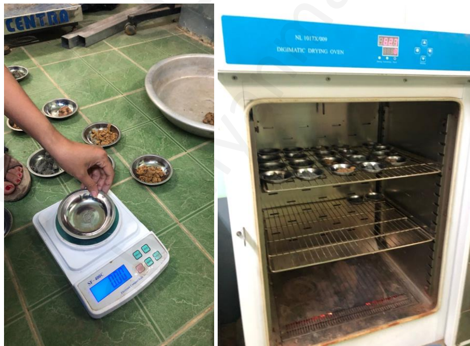
Figure 65: Moisture Testing of Samples
