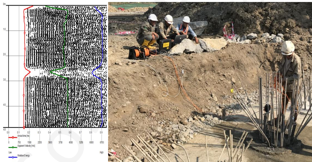
Figure 5: Waterfall Reflectogram; Sonic Logging Testing on Bored Pile
