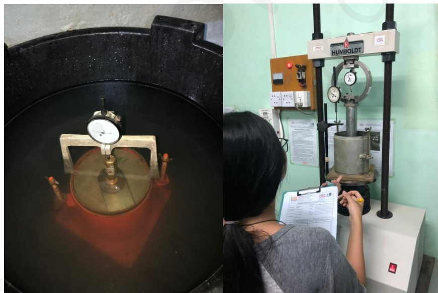
Figure 84: CBR Testing Photos
