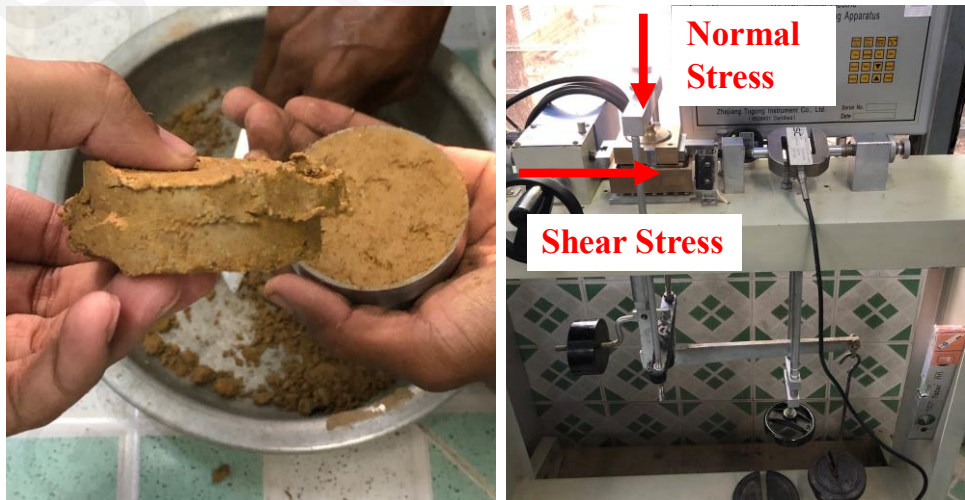
Figure 73: DS Tested Sample, Sample Preparation and Shearing Apparatus
