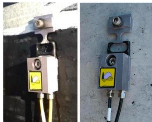
Combined sensors to be used on both steel and concrete piles, easy to mount with two bolts
