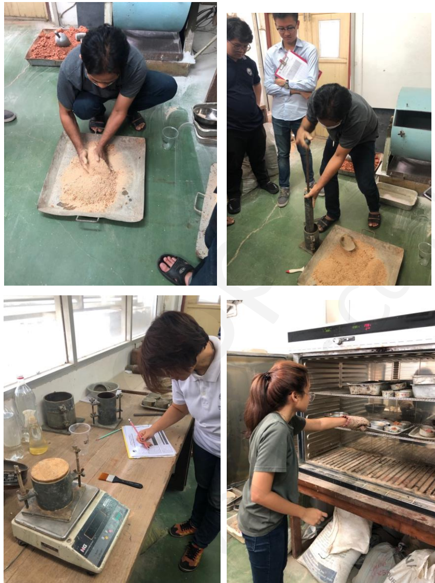
Figure 82: Compaction Testing Photos
