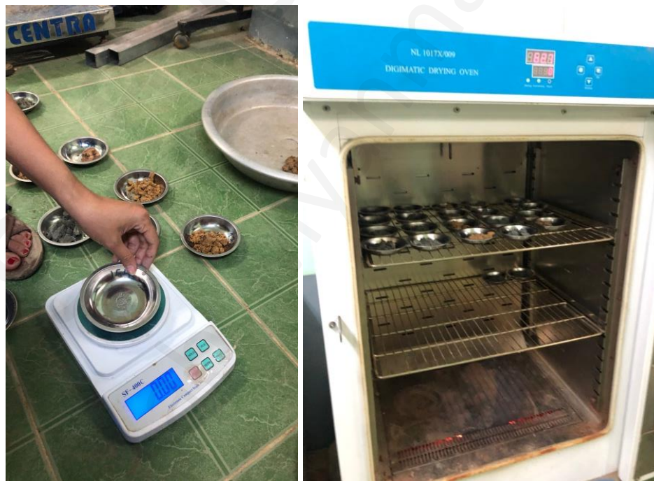
Figure 65: Moisture Testing of Samples
