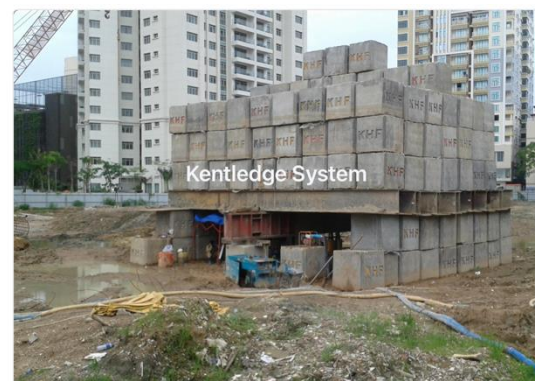
Figure 18: GEOLAB's Inverted Beam System & Kentledge System
