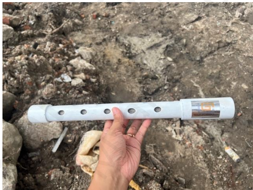
Figure 31: Casagrande Piezometer & VW Piezometers
